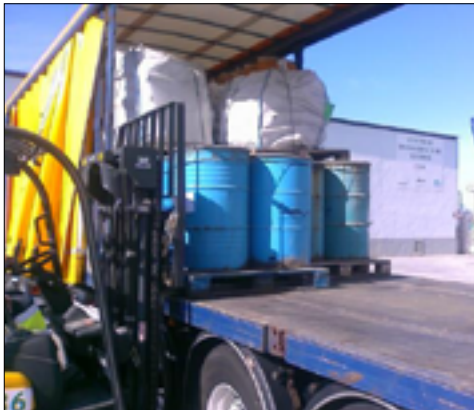
Detail of works to load containers containing HW to trailer for subsequent unloading at a final destination plant.
