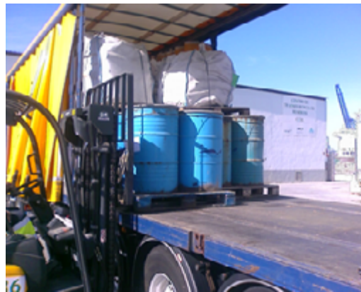
Detail of works to load containers containing HW to trailer for subsequent unloading at a final destination plant.
